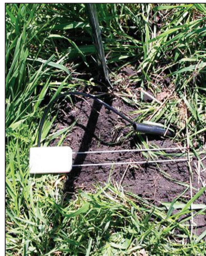
Figure 6. Campbell Scientific CS616 soil moisture probe
